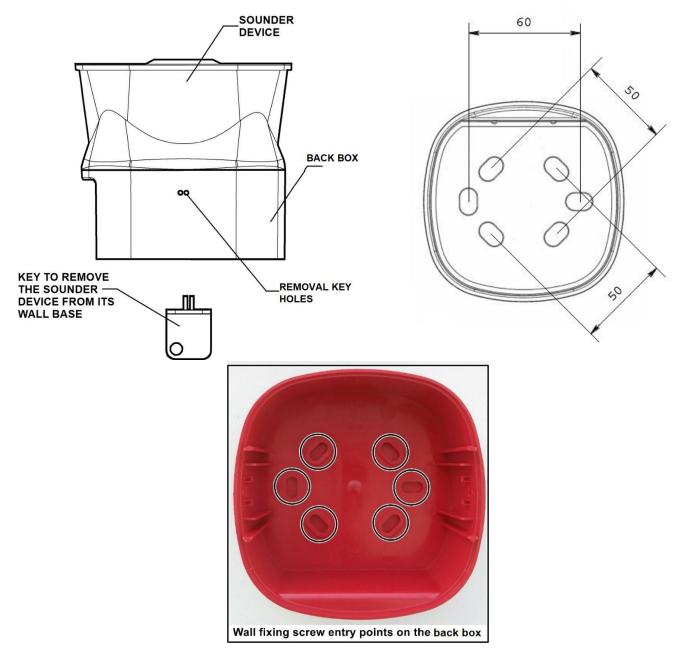
Preferably, the device should be installed away from metallic objects, doors, and power lines, as they can cause the communication distance to drop. It is also important to avoid installing the device near electronic and computer equipment in order to protect it from potential electromagnetic interference.
